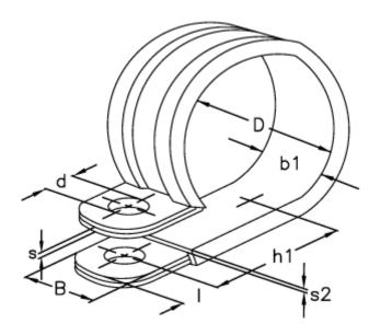
$\begin{array}{lll} \text{b1} & = 15.0 \\ \text{d} & = 5.3 \\ \text{Diameter D} = 69 \\ \text{h1} & = 42.5 \\ \text{I} & = 5.0 \\ \text{s} & = 0.50 \\ \text{s2} & = 1.2 \\ \text{Width B} & = 12 \\ \end{array}$
